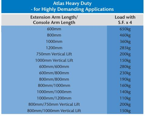
BeaconMedæs pendant systems have been tested to 40,000 revolutions under the maximum loads shown with a safety factor of 4, ensuring faultless reliability. Other manufacturers may use alternative methods of calculation, such as applying a safety factor relating to catastrophic failure of the pendant system. This method is less stringent and does not provide an accurate comparison with the products described herein.
